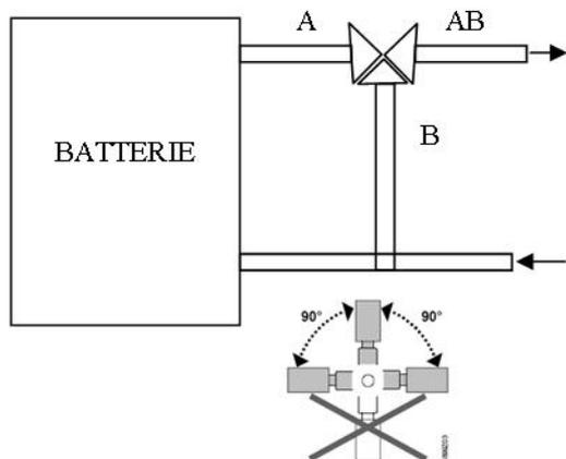
**LA VANNE DOIT ETRE RACCORDEE HORS TENSION**
